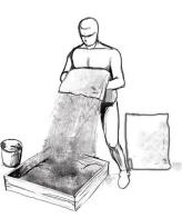
Add 2 clean sand bags previously strained., then mix it up with the cement to get an homogenously mixture. Sand works like an aggregate.
