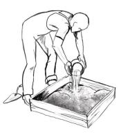
*Place* 5 gallons or 1 big bucket of water to the mixture. Water will join the hole mixture.
